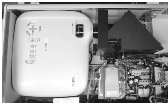
Figure 7: iLight 3D system showing projector, camera, and optical box including half-mirror and optical trap.
